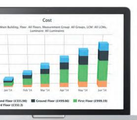
The company's facilities management team wanted to quantify the reductions in energy consumption, to justify the cost of the swap-out. CP Electronics' RAPID energy measurement devices were installed to monitor the energy consumption of the light fittings, and following the retrofit, the client found active energy consumption reduce from 687w per day to 221w per day in this area – a 67% reduction in energy usage.
