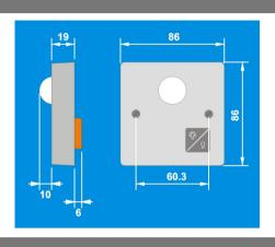
The PDS presence detection switch replaces a standard single gang light switch. It detects movement using a PIR sensor and turns the lights on, (either incandescent and fluorescent loads). An internal light sensor is provided for additional energy saving. When an area is occupied lighting is only switched on when the level of natural light is below a preset level. When an area is no longer occupied the lights will switch off after an adjustable time out period.
