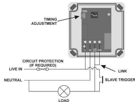
Diagram 2 Wiring for three wire switching circuits
