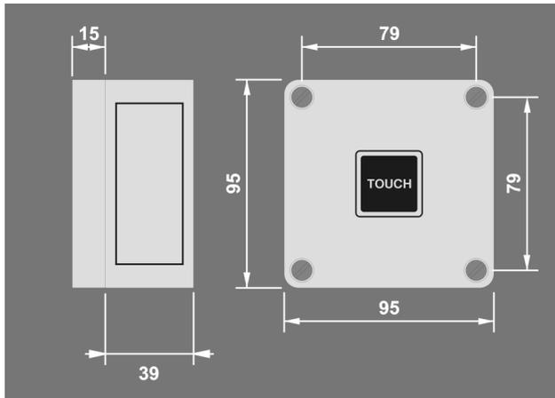
The MRT16 series of time delay switches are designed to provide timed control of lighting, heating or ventilation loads. Using touch (light press required) activation the user can switch on a load for a preset time period and have the load turn off automatically after the time period has elapsed.
