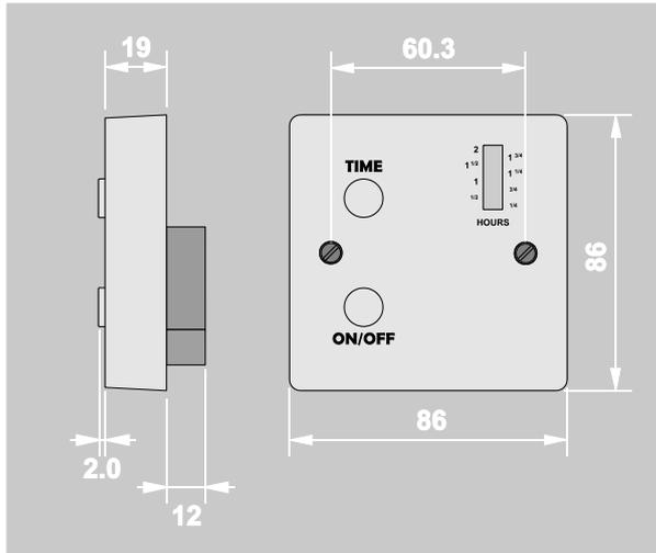
The RBT1 run back timer is a high output electronic timer which provides control for a wide range of loads. Its powerful 20A output makes it particularly suitable for the control of immersion heaters. The unit allows an appliance to be powered for a set time period which can be adjusted by the user. A simple display shows the user how much time is left to run. An ON/OFF switch allows the user to cancel the timing program whilst a memory remembers the last timing sequence selected.
