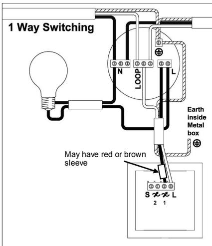
If the lights are controlled from one location only, wire as in the diagram.
