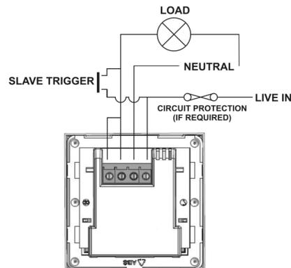
Diagram 2 Wiring for three wire switching circuits
