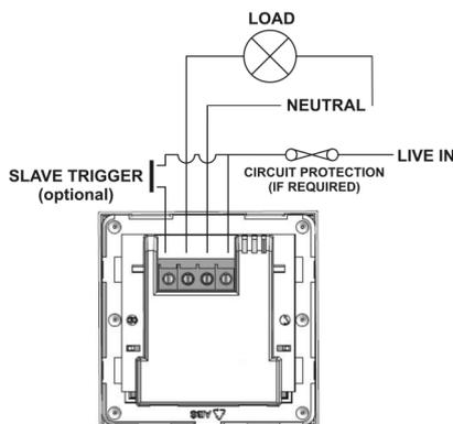
Diagram 1 Standard Wiring
